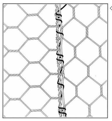
The ends of the diaphragms must now be permanently laced to the sides of the mattress with single loops and double loops in turn at every second mesh interval.
