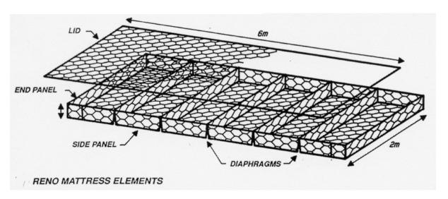
**2.** Flatten out each mattress in a hard, flat surface, and stamp out unnecessary creases. Creases will have to be stamped into the bottom of the 2nd and 4th diaphragms.
