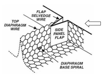
**3.** Ensure that each diaphragm is vertical and the correct height. Fold the sides and ends of the mattress to meet the top of the diaphragms.
