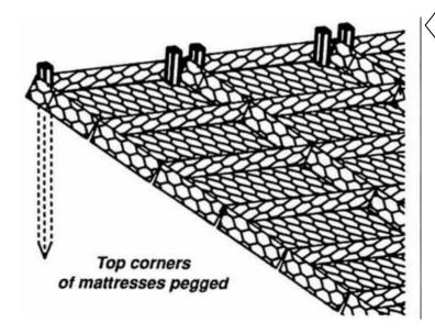
Generally, when the mattress is being installed on a slope steeper than 1 in 1.5 or on soft or sandy slopes it should be secured by star pickets or hardwood pegs driven into the ground just inside the upper end panel, at 2.0 centres or as necessary.
