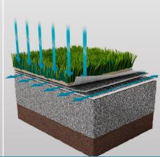
2 in 1: MacSport combines drainage-enhancing action with shock absorption functions
