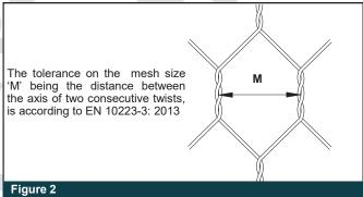
A PoliMac<sup>®</sup> coating with a nominal thickness of 0.50 mm is then applied to provide added protection for use in hydraulic works, polluted environments or wherever the risk of corrosion is present. The standard specifications of mesh-wire are shown in
