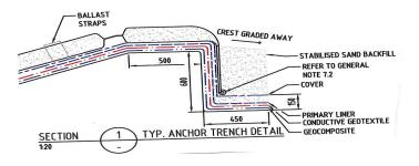
Cross-section of lining system, showing conductive geotextile under primary liner but above the geocomposite drain
