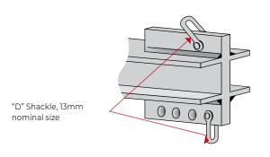
Figure 4. Spreader Bar
